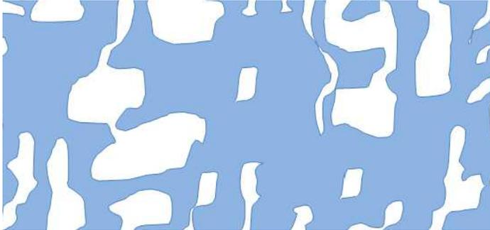
**NOTE:** The white spaces are voids in the material which will allow liquid to penetrate.
