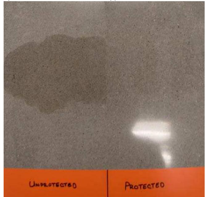
**NOTE:** The above picture shows the stain left from exposure of concrete to motor oil with a 20 minute dwell time. Note the protected side resisted the motor oil while the unprotected side resulted in a stain.
