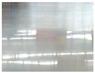
**NOTE:** In this image the concrete toward the front has a 60° gloss of 16.3 and a DOI of 80.9 with clearly reflected overhead lighting. The area in the rear has a 60° gloss of 16.4 and a DOI of 27.5 with overhead lighting visible only as a blur.
