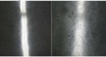
NOTE: The flooring on the left in the above picture was prepared using 3M™ Trizact™ Diamond TZ Abrasive Pads and has a 60° gloss of 78 and a DOI of 71. The flooring on the right was not prepared with 3M™ Trizact™ Diamond HX Discs and has a 60° gloss of 74 and a DOI of 43.
