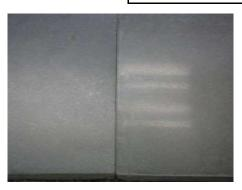
**NOTE:** The above picture shows two uncoated concrete tiles with similar 60° gloss (42 left and 49 right) but a different DOI (27 left and 75 right). Notice how the reflected lights are clear in the right hand tile and only a blurred image in the left tile
