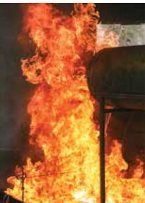
Fire Performance Engine Test: Fuel flows from a jet engine nacelle mock-up and feeds a pool fire.
