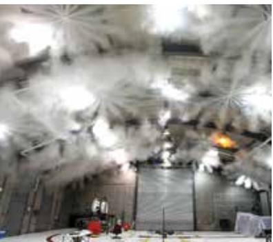
Concentration Test: 3M™ Novec™ 1230 Fire Protection Fluid is discharged in the Dannelly Field hush house.
