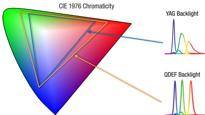
Figure 3. The color gamut produced by a display with a quantum dot-equipped backlight can be approximately 50 percent larger than the gamut produced by the same display with a conventional white YAG LED backlight.
