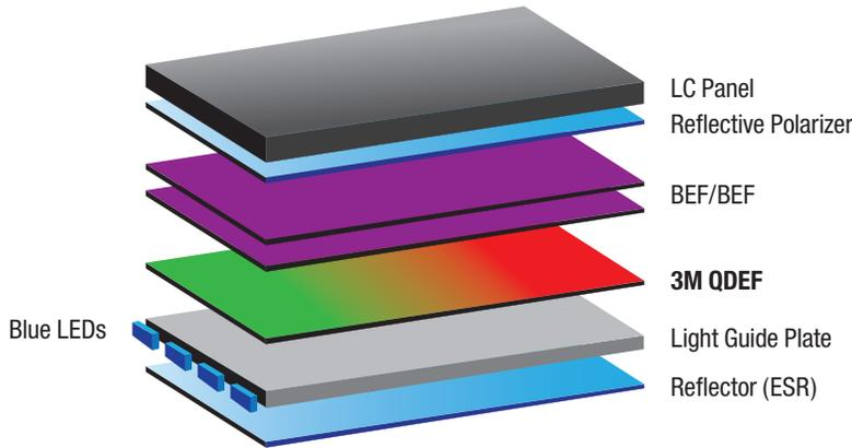
**Figure 7. Introducing 3M QDEF is minimally disruptive to typical LCD architecture. Because 3M QDEF has diffusive properties, it can replace the current diffuser film in a backlight unit (as shown here) while other components remain in place. The only other significant mechanical change required is the replacement of traditional white LEDs with blue LEDs.**
