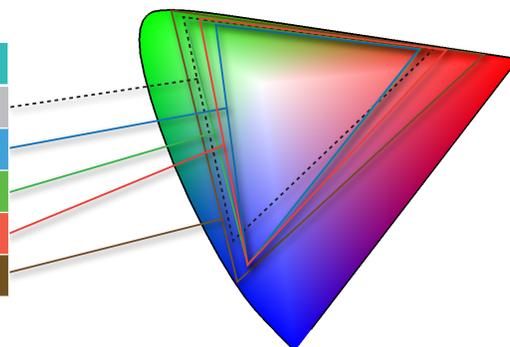
Figure 5. Various color gamuts relative to the CIE 1976 Chromaticity Diagram.
