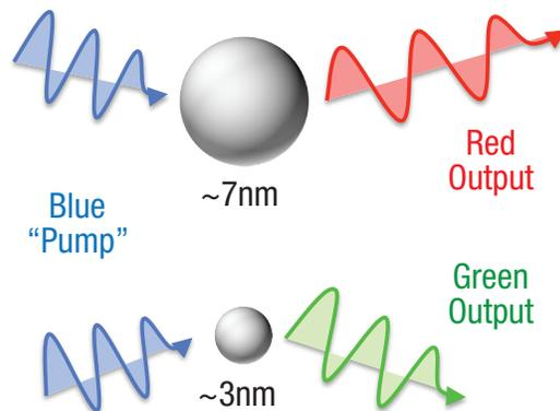
Figure 1. When struck by blue photons, 7-nm quantum dots produce red light and 3-nm dots produce green light.
