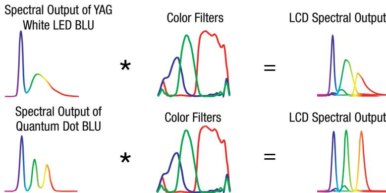
Figure 2. When the light from a conventional “white” YAG LED passes through a color filter, the greens and reds appear unsaturated. When light from an LED is converted by quantum dots instead of a yellow phosphor, it has concentrated peaks and final colors are saturated.
