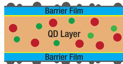
Figure 6. 3M QDEF construction: a stack of two barrier films and a film of quantum dots dispersed in a polymer matrix.
