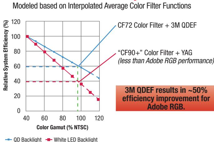
**Figure 8. Modeling analysis showing relative LCD system efficiency. The Adobe RGB color gamut can be achieved using 3M QDEF or highly saturated color filters; the 3M QDEF displays are approximately 50 percent more efficient than displays using the more saturated (CF90+) color filters.**
