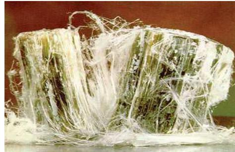
materials to give a hard, durable product e.g. mixed with resin to make a fireproof composite board (like Lebah, Zelemite) or when mixed with cement to form fibro type sheeting, asbestos cement pipes etc.
