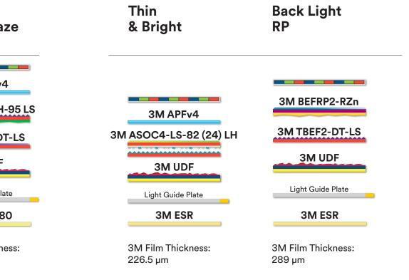
3M<sup>™</sup> Advanced Polarizer Film-Quarter Wave Plate (APF-QWP) 3M<sup>™</sup> Advanced Polarizer Film (APF) 3M<sup>™</sup> Brightness Enhancement Film Reflective Polarizer (BEFRP) 3M<sup>™</sup> Advanced Structured Optical Composite (ASOC) 3M<sup>™</sup> Thin Brightness Enhancement Film (TBEF) 3M<sup>™</sup> Ultra Diffuse Film (UDF) 3M<sup>™</sup> Advanced Specular Reflector (ASR) 3M<sup>™</sup> Enhanced Specular Reflector (ESR) 3M<sup>™</sup> Enhanced Diffuse Reflector (EDR)
