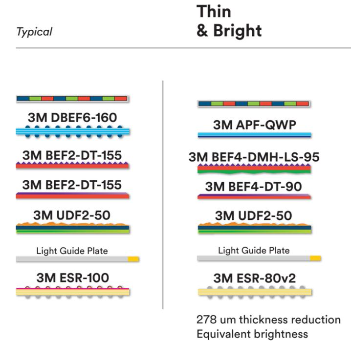
278 μm thickness reduction
