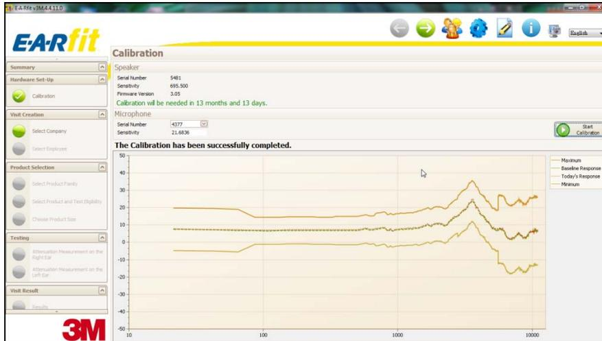
Speaker serial number, sensitivity and firmware version will be automatically detected by the software. The software will also detect when your speaker is due for its factory calibration. The “calibration due date” message will change from green to yellow to red depending on how close you are to the calibration due date.
