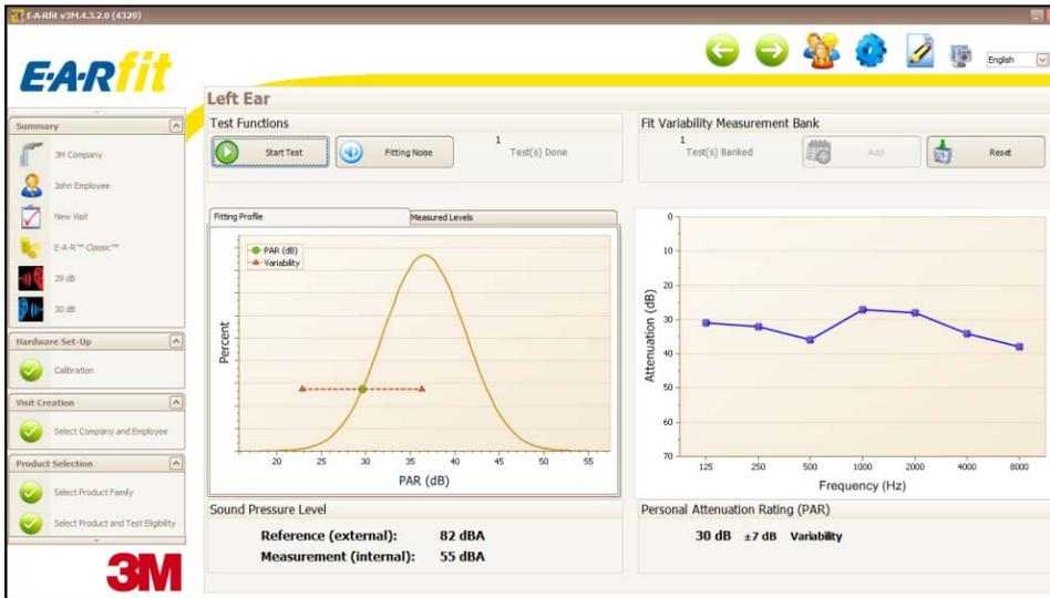
At the completion of the test for each ear, the results are displayed on this screen. You will have the option to bank or “Add” the test to the “Fit Variability Measurement Bank” before continuing. This bank is specific to this test subject.
