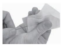
Note: Use clean areas of the lint-free wipe; try not to wipe fibers more than two times. Limit stripped fiber exposure to the atmosphere to one hour or less.
