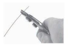
Note: The strip tool should be clean and in good operating order to prevent damage to the glass cladding.
