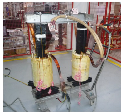
Two identical 75 kVA coils; One with 3M™ Insulation and one with calendered meta-aramid
