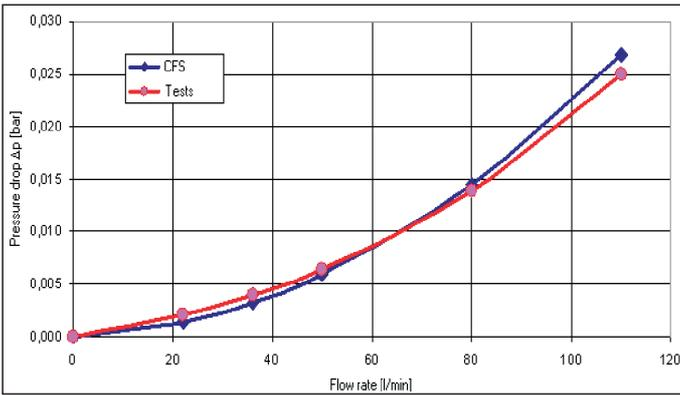
Fig. 9 Comparison of CFS and flow test results
