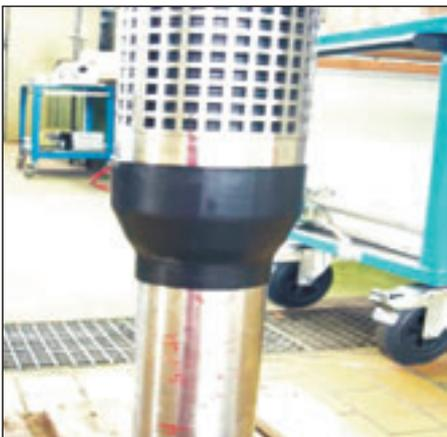
Fig. 7 Example of a Polyolefin shrinking hose
