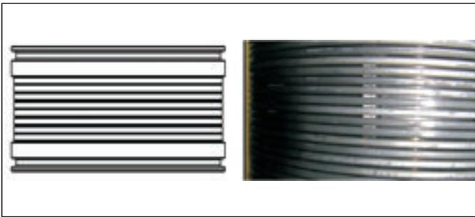
Fig. 5 Stack of ceramic screen elements, left: engineering drawing, right: picture of stacked rings, gap width 320 µm
