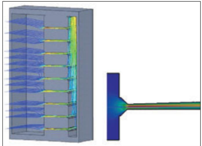
Fig. 8 CFS data for flow rates of 80 m<sup>3</sup>/d and a gap width of 250 µm, left: flow lines along the screen; right: gap velocity plot (blue = low velocity, red = high velocity)
