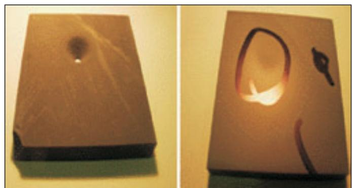
Fig. 4 Porous versus solid ceramics (both samples SiC) after sand blasting
