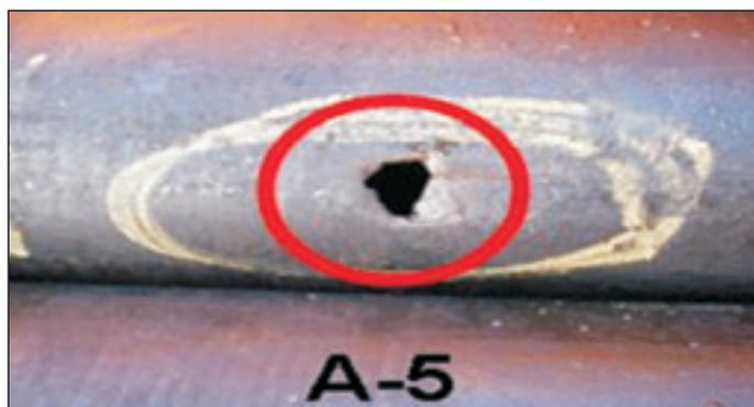
Fig. 3 Eroded pipe
