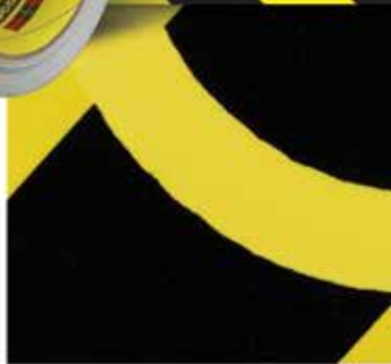
Competitive Safety Stripe Tape After 1,000 abrasion wear cycles, the color black is worn away.
