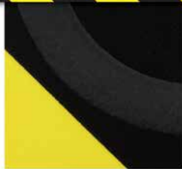
3M™ Safety Stripe Tape 5702 After 1,000 abrasion wear cycles, the black color is still visible.
