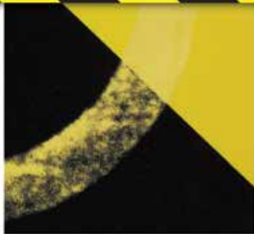
Competitive Safety Stripe Tape After only 25 abrasion wear cycles, the black color is wearing away quickly.
