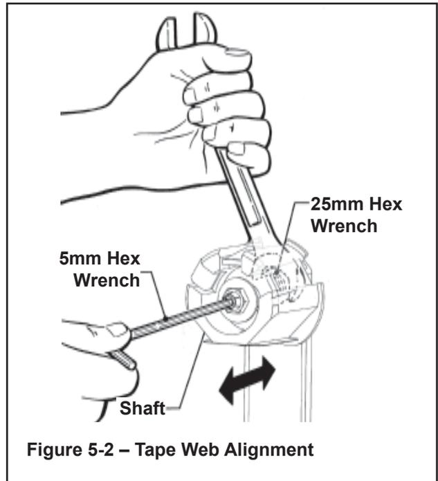
**Figure 5-2 – Tape Web Alignment**
