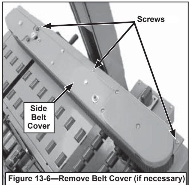
**Figure 13-6—Remove Belt Cover (if necessary)**
