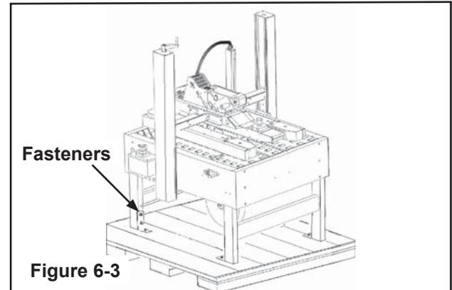
Remove the leg height adjustment cap screws and replace with the cap screws from the tool kit. Loosen both cap screws. Remove and replace them one at a time to keep the inner threaded plate in position.
