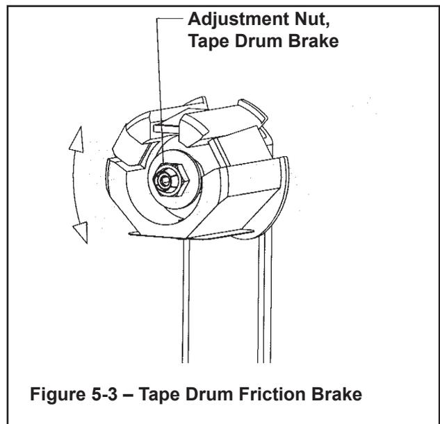
**Figure 5-3 – Tape Drum Friction Brake**
