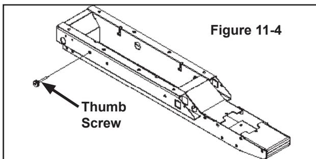
3. Slide head forward and lift upward to remove
