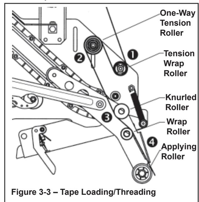
**Figure 3-3 – Tape Loading/Threading**
