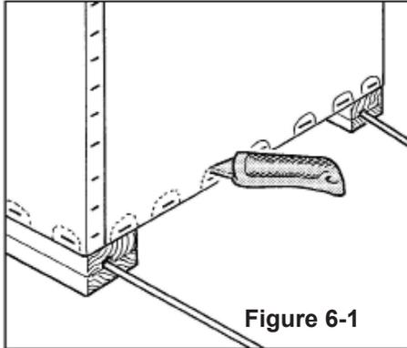
After cutting out or removing the staples, lift the shipping box in order to clear the machine
