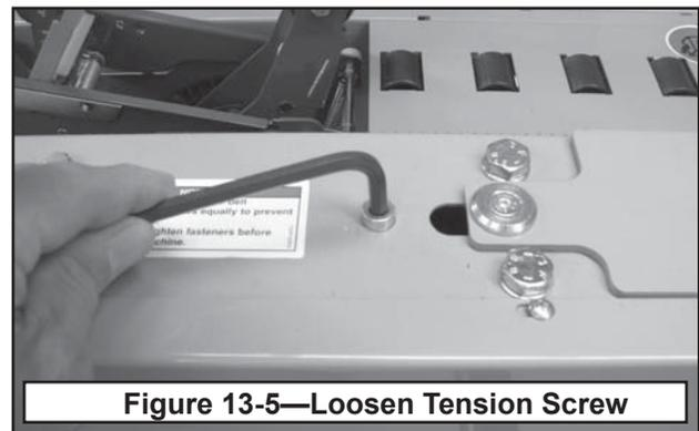
**Figure 13-5—Loosen Tension Screw**
