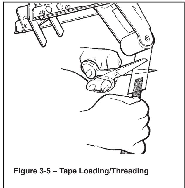
**Figure 3-5 – Tape Loading/Threading**
