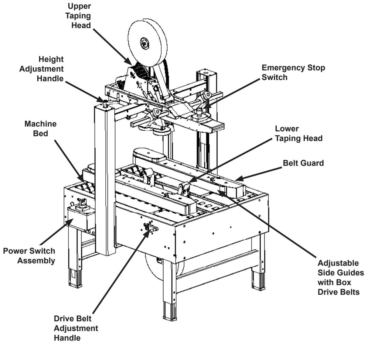
**Figure 3-9—**a80/a80-3 Case Sealer Components (Left Front View)
