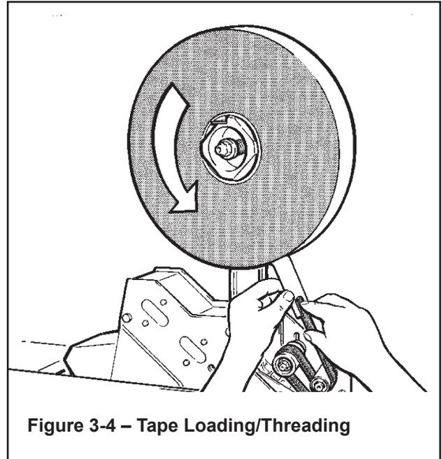
Figure 3-4 – Tape Loading/Threading
