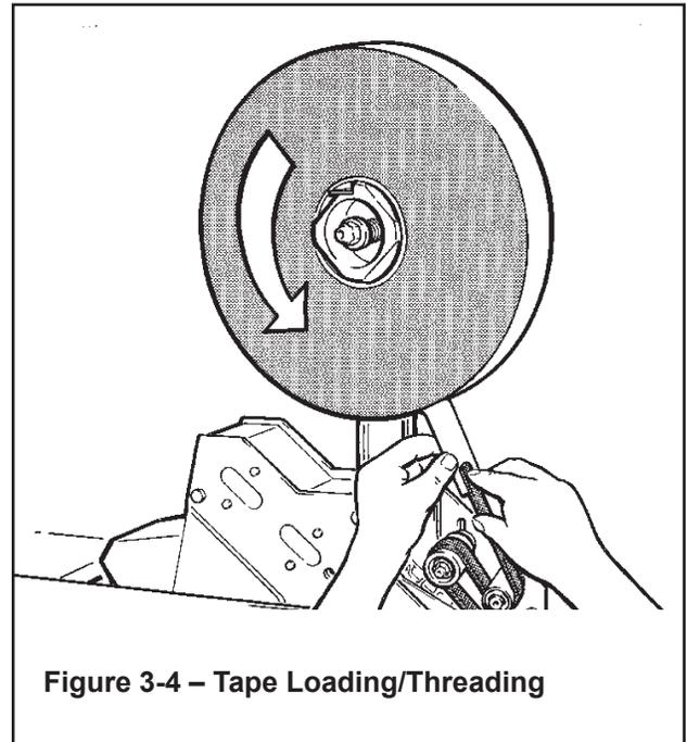
**Figure 3-4 – Tape Loading/Threading**
