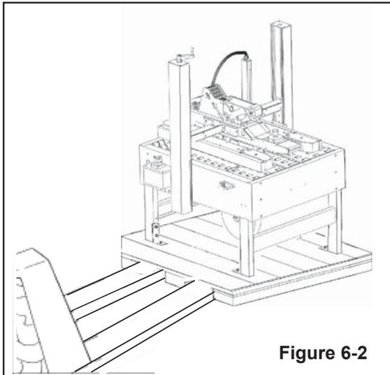
Transport the machine with a fork-lift truck to the operating position. Lift the pallet at the point indicated in **Figure 6-3** (weight of machine + pallet = see **Section 4**).
