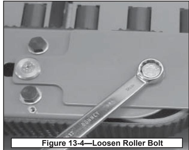
**Figure 13-4—Loosen Roller Bolt**
