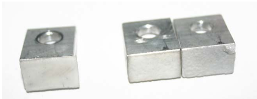
Figure 16: Quasi-static sample (left) and high rate sample (right) after test.
