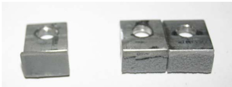
Figure 11: Quasi-static sample (left) and high rate sample (right) after test.
