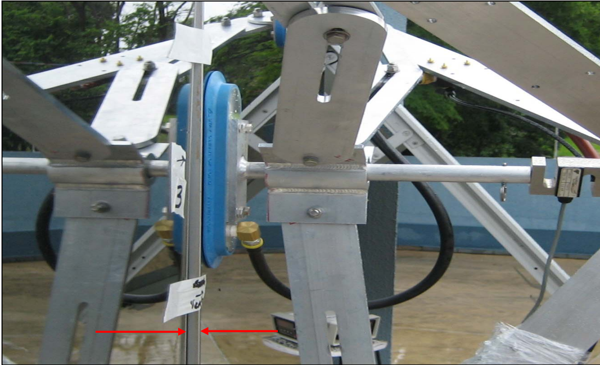
Photo #020: Blow-up photo of glass / framing offset due to testing (pulling action) being performed.
