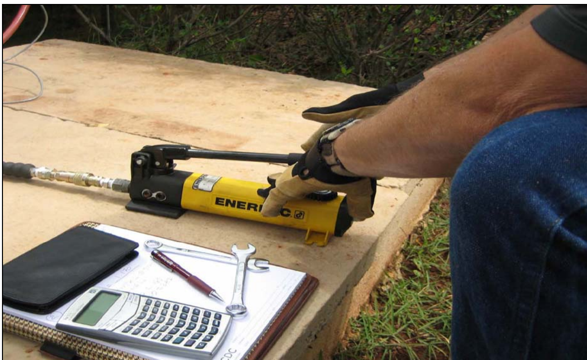
Photo #003: Hydraulic pump which is connected to the hydraulic cylinder on the test apparatus. The pump operator monitored the pressure meter, keeping it at the desired load.
