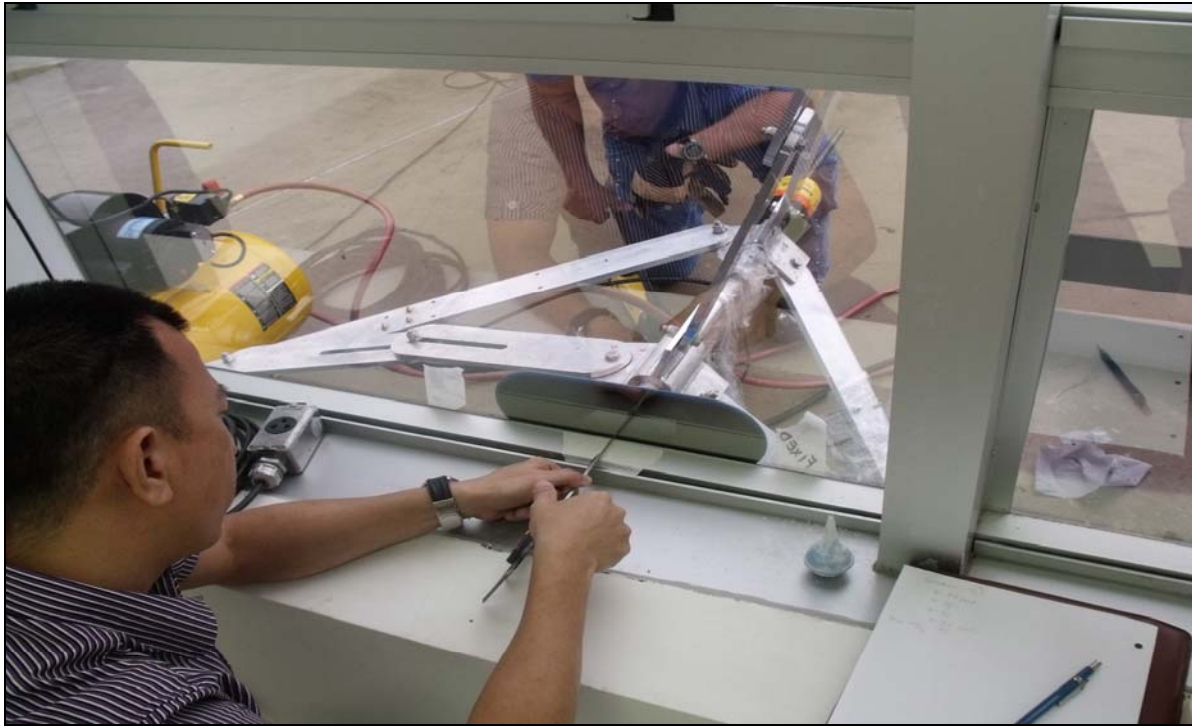
Photo #005: Prior to testing, the distance from the inside face of glass to a surface on the aluminum framing is measured (if possible) in its original state of rest using calipers. During each test, the displacement of the glass relative to the aluminum framing is also measured and recorded.
