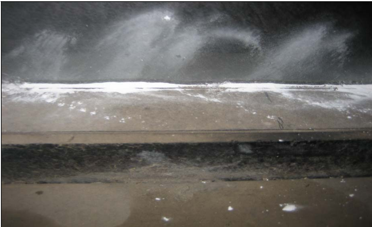
Photo #006: Talcum powder was applied at the interior 45 seconds into the overload test to determine if there was evidence of adhesion failure of the VHB SGT to the glass. If adhesion failure occurred, powder would fall into the detached area or void, producing an uneven line of powder when viewed from the exterior (See Photo #007 for exterior view).
