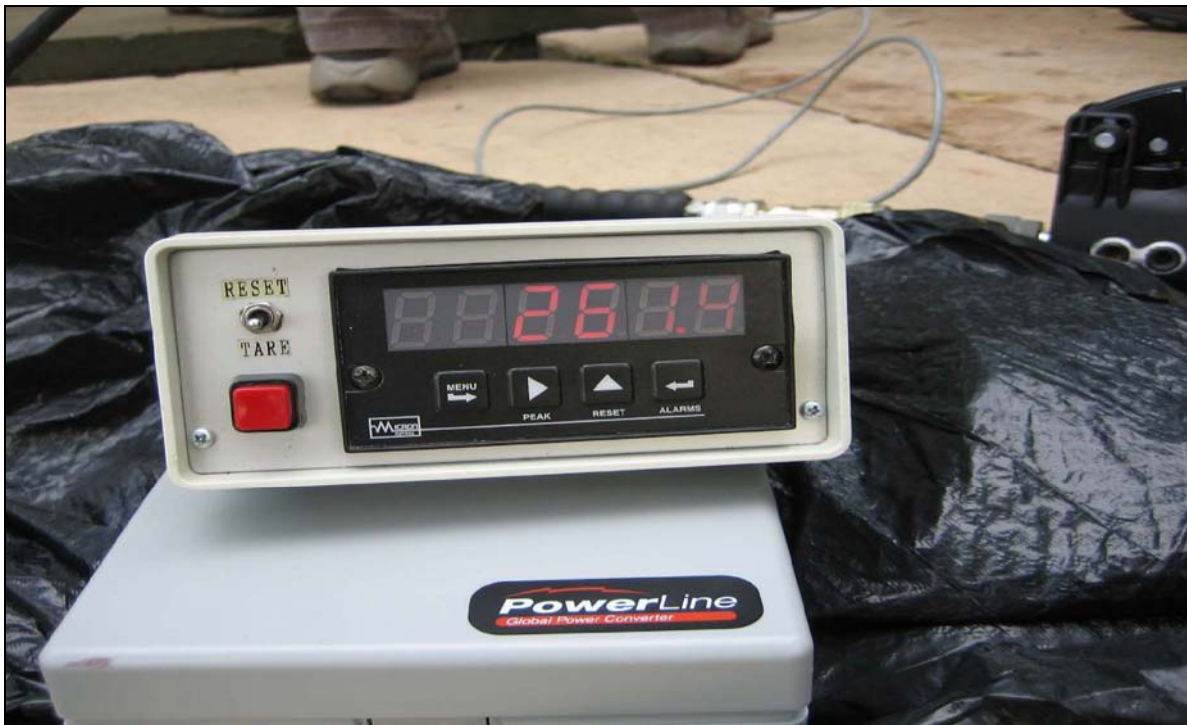
Photo #004: The pressure meter connected to the load cell was monitored, keeping the desired force being pulled on the vacuum pad. "S"-Type Load Cell & Pressure Meter were calibrated by RECAL on 11/29/2010 (See Certificate of Calibration attached to this report).
