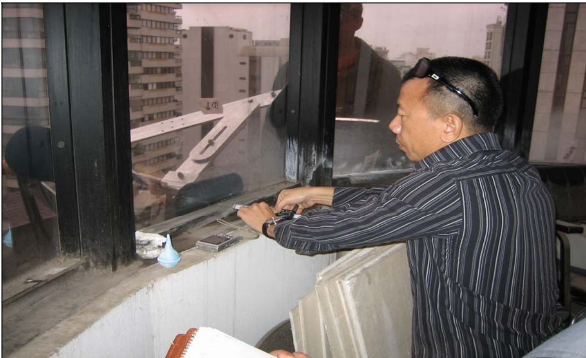
Photo #021: During each test, the displacement of the glass relative to the aluminum framing is measured and recorded.
