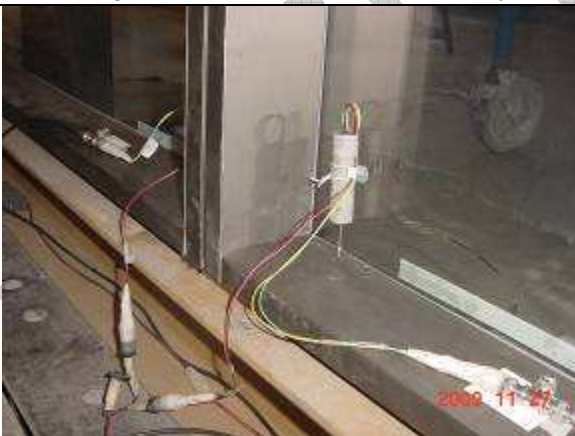
Photograph 3.5: Detail of the central located transducer for vertical displacement measurement of the aluminum frame bottom profile. West side.
