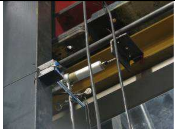
Photograph 3.2: Detail of the sample total horizontal displacement measuring transducer.
