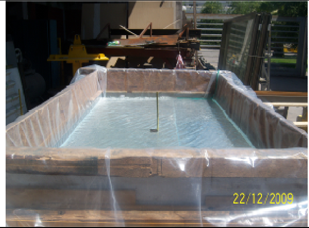
Photograph 4.10: General view of the emptying test (filled pool) to laminated glass system module.
