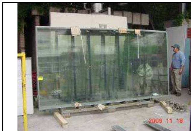
Photograph 2.2: General view of the module with the aluminum perimetric frame.
