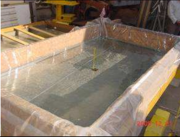
Photograph 4.9: General view of the emptying test (filled pool) to thermo-panel system module.
