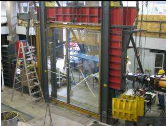
Photograph 3.1: General view of the wall curtain system cyclic shear test implementation.
