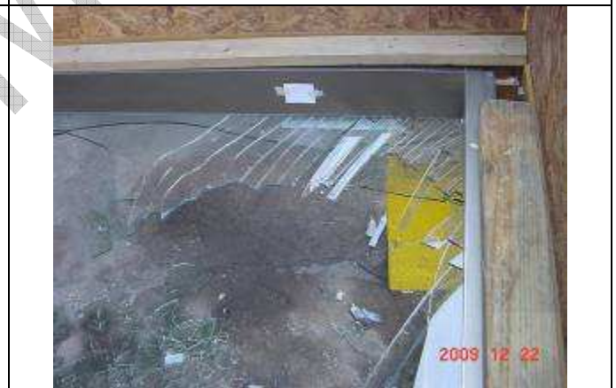
Photograph 4.12: General view of the final condition of thermo-panel module subjected to emptying test.
