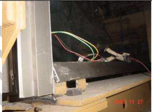
Fotografia 4.8: Details of the bottom east horizontal profile break of the of aluminum frame of the module with the laminated glass, in the 50mm cycle of the sample 2
