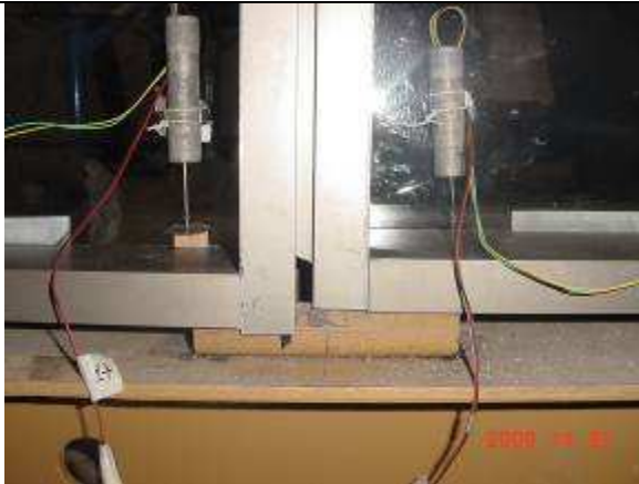
Photograph 4.7: Details where the small break is shown of one of the aluminum profiles in the bottom central sector of sample 2
