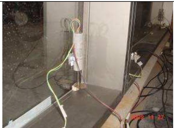
Photograph 3.6: Detail of the central located transducer for vertical displacement measurement of the aluminum frame bottom profile. East side.
