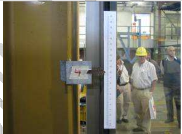
Photograph 3.4: Detail of one of the graduated rulers used to measure displacements in tests
