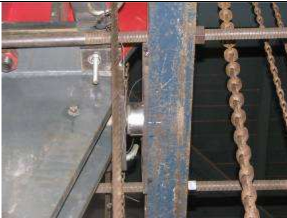
Photograph 3.3: Detail of one of the load cells implemented for the registration of the load applied to the system.
