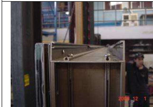
Photograph 2.4: Geometry detail of the aluminum frame vertical profile that is located in one of the module ends.
