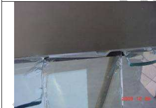
Photograph 4.13: Detail of one of the borders, where it is possible to observe a segment of elongation of the 3M tape, concluded the thermo-panel module emptying test.
