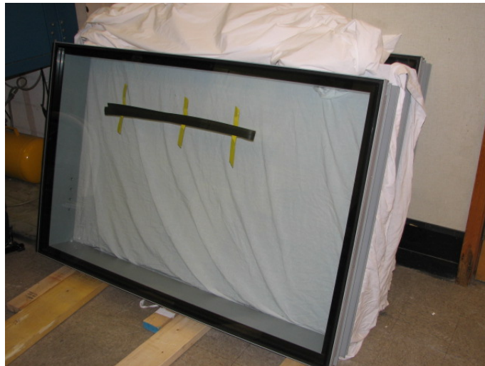
Figure 9- Smaller Unitized System Panel (Exterior View)
