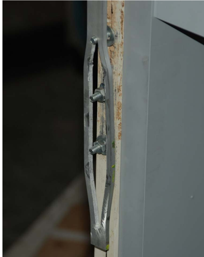
Figure 34- Extent of Slotted-Hole Widening
