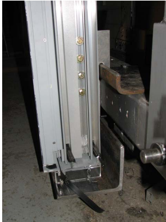
Figure 7- Attachment of the Bottom of the Specimen to the Facility
