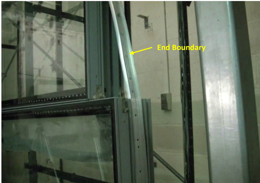
Figure 28- End Boundary Acting as a Tension Member
