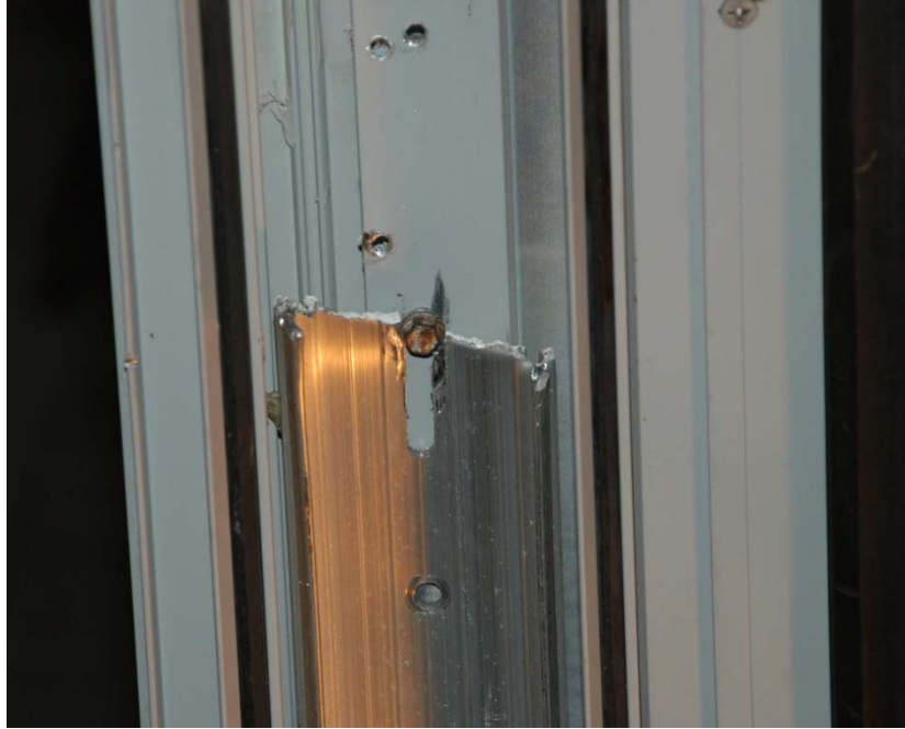
Figure 36- Sheared Boundary Element
