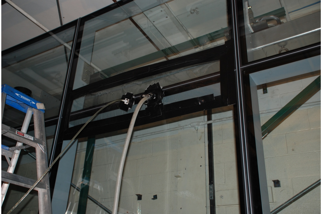
Figure 38- Typical Shroud for Air Leakage Tests
