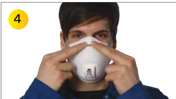
4. Using both hands, mould nose clip to the shape of the nose bridge by pushing inwards while moving your fingertips down both sides of the nosepiece.
