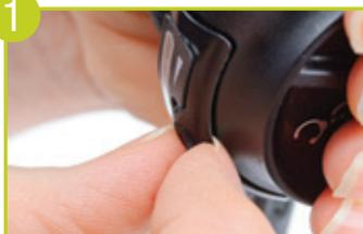
Place pointer finger between Control Pod and Battery; place thumb on the battery latch.
