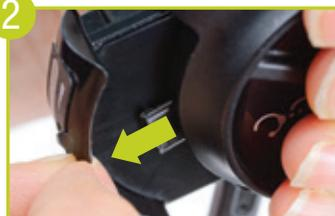
Using a pinching motion, pinch and gently pull battery straight out.
