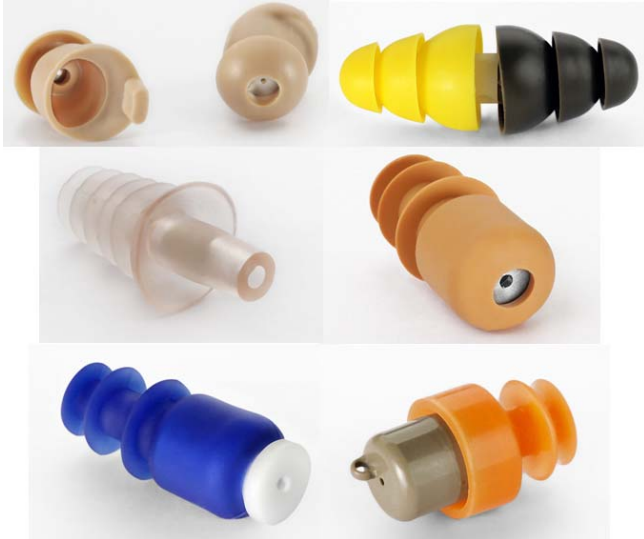
Figure 3 – Earplugs tested in this study as described in Table 1. Gunfender (back and front view), Combat Arms, Noise Braker, Ear Valvs, Sound Baffle, and Quiet Please (left to right, top to bottom).
