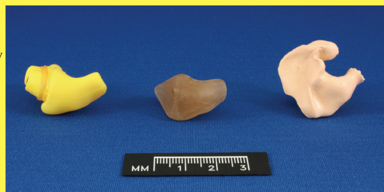
A custom earplug made with the inflatable-bladder technique (left), a laboratory-finished earplug (center), and a mold-in-place custom earplug (right).
