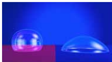
Water drop on Aquasil Impression Material prior to set (left). Initially, Aquasil shows hydrophobic behavior. Water drop on Impregum™ Soft Polyether Impression Material prior to set (right).
