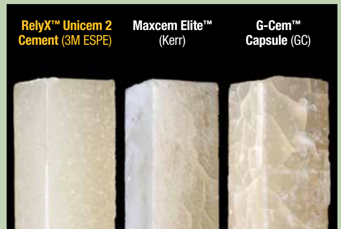
Results of stress test on self-adhesive resin cements. Specimen 2 x 2 x 25 mm self cured (according DIN ISO 4049:2000) after 10,000 thermocycles (at 10 days) in water 5°/55°C (with 30 seconds dwell time). Source: 3M ESPE internal data.
