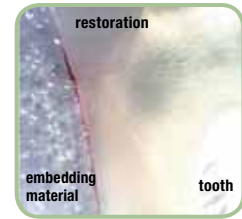
Fig. 12: RelyX™ Ultimate sample of dye penetration test, no penetration of fuchsine solution into dentin or interface.
