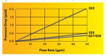
**Pressure Drop:**  $3M^{\infty}$  500 Series High Performance Filter Bags have low initial pressure drop ( $\Delta P$ ) in water as the chart indicates. The chart includes the pressure drop of a typical single vessel to assist filter system sizing.
