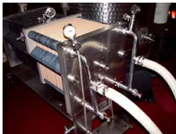
**Figure 2—Typical Filter Press or Sheet Filter**
