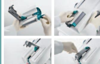
Insert the Penta<sup>™</sup> Foil Bags with your desired 3M ESPE impression material into the cartridge. Then place the cartridge in the Pentamix<sup>™</sup> Lite Mixing Unit and attach a Penta<sup>™</sup> Mixing Tip - Red. Mixing and dispensing starts at the press of the green start button. Now, directly fill the impression tray or syringe with the homogeneously mixed impression material.
