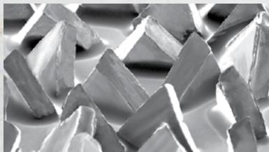
3M precision-shaped grains are electronically oriented to form sharp peaks that easily “slice” through metal. They stay cooler, cut faster and last longer.
