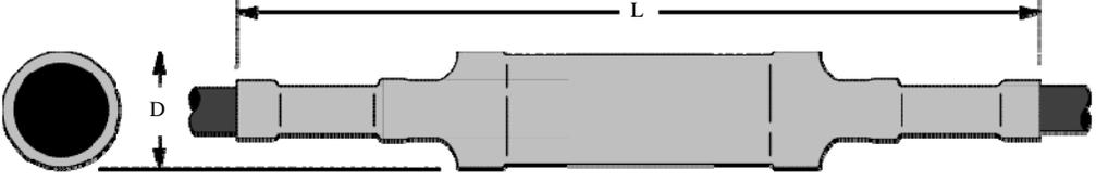
The diagram shows a side view of the splice kit with a dimension line labeled 'L' indicating the total length and a dimension line labeled 'D' indicating the diameter of the central body. A circular inset shows the end view of the splice.
