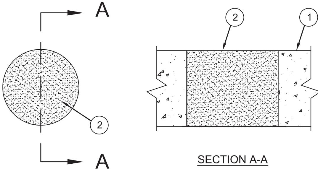
1. **Floor or Wall Assembly** – Min 2-1/2 in. (64 mm) thick lightweight or normal weight (100-150 pcf or 1600-2400 kg/m<sup>3</sup>) concrete. Max diam of opening is 8 in. (203 mm).
