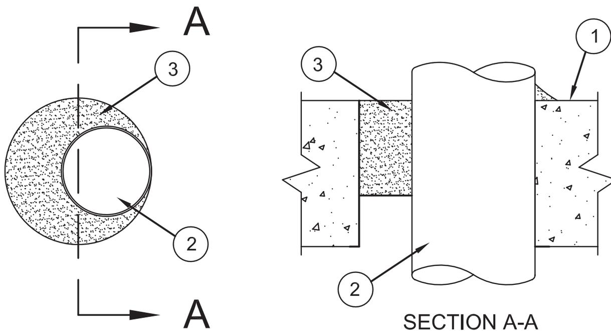
1. **Floor or Wall Assembly** – Min 2-1/2 in. (64 mm) thick lightweight or normal weight (100-150 pcf or 1600-2400 kg/m<sup>3</sup>) concrete. Max diam of opening is 12-1/2 in. (318 mm).
