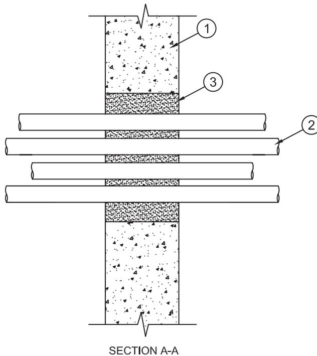
1. **Wall Assembly** – Min 6 in. (152 mm) thick reinforced lightweight or normal weight (100-150 pcf or 1600 - 2400 kg/m<sup>3</sup>) concrete wall. Wall may also be constructed of any UL Classified **Concrete Blocks\***. Max area of opening is 720 in<sup>2</sup> (4645 cm<sup>2</sup>) with max dimension of 30 in. (762 mm).
