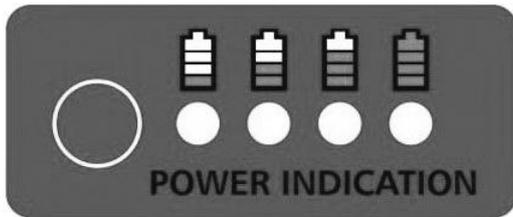
The Battery Pack has a “SW” button and 4-step green LEDs for indicating remaining capacity status and Over temperature condition.
