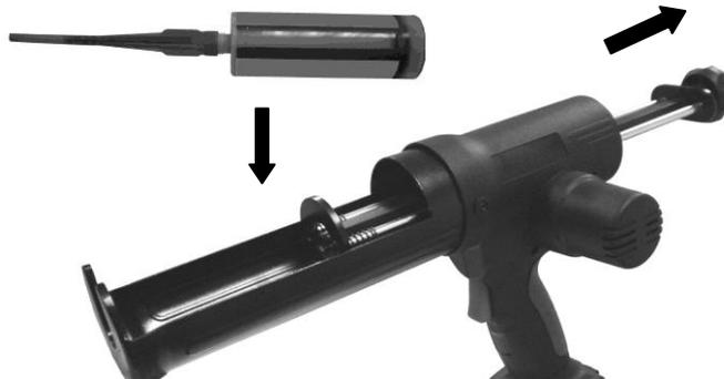
4. Push the rear knob to have the disk slightly contact with cartridge to start operating the epoxy gun.
