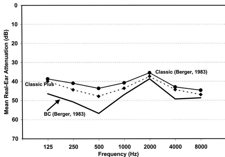
FIG. 3. Comparison of the real-ear attenuation of a deep insertion of the Classic Plus (this study) to the Classic, and to the BC limits, from Berger (1983).
