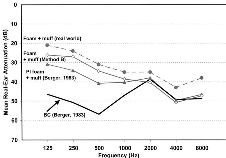
FIG. 12. Comparison of laboratory-estimates of the BC limits versus the actual protection in the real world for a foam plug plus small earmuff.
