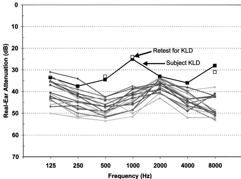
FIG. 5. Real-ear attenuation for foam plugs with a deep insertion (DI). Each line represents the average of two measurements on one subject. The “aberrant” subject KLD is specifically noted.
