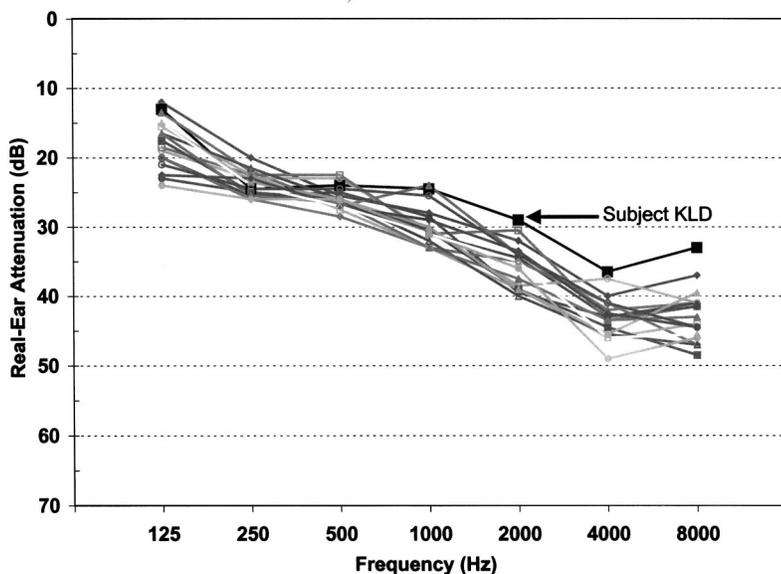
FIG. 6. Real-ear attenuation for ANR earmuff with the ANR off. Each line represents the average of two measurements on one subject. The “aberrant” subject KLD is specifically noted.
