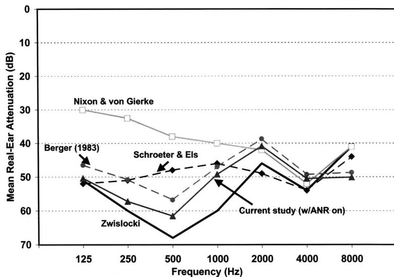
FIG. 10. Various estimates of the BC limits to attenuation with head exposed, from this study and the prior literature.
