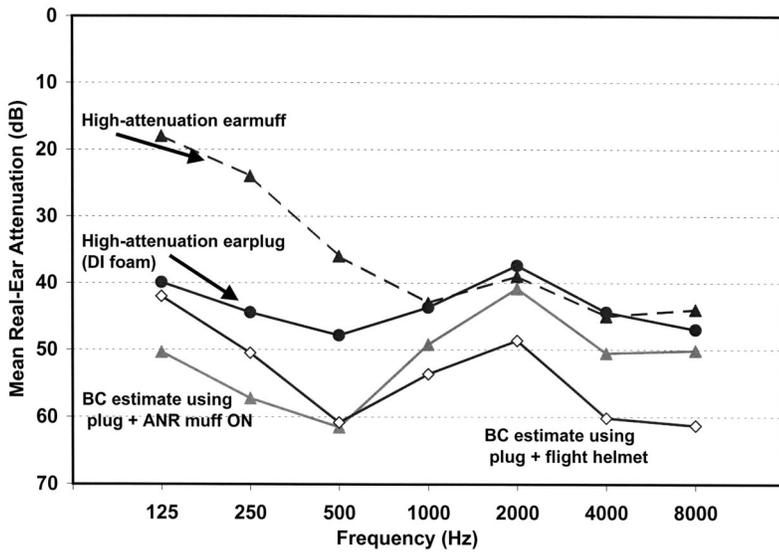
FIG. 9. Various estimates of the BC limits with head exposed versus covered, from the current study.
