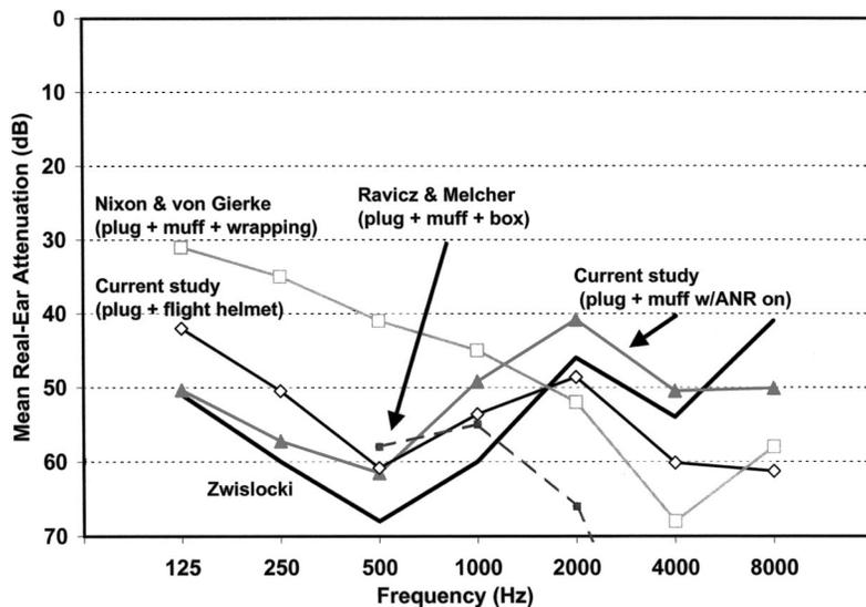
FIG. 11. Various estimates of the BC limits to attenuation with head exposed versus covered from this study and the prior literature.
