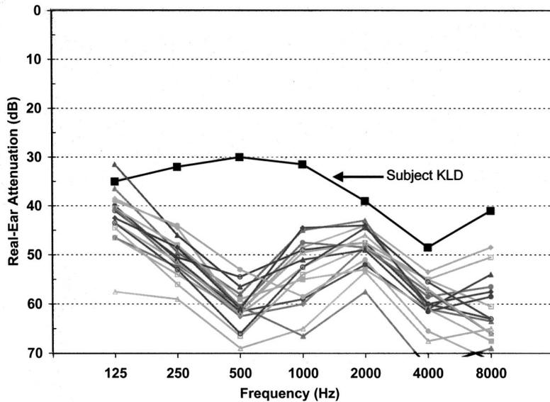
FIG. 7. Real-ear attenuation for foam plugs with deep insertion (DI) plus flight helmet. Each line represents the average of two measurements on one subject. The “aberrant” subject KLD is specifically noted.
