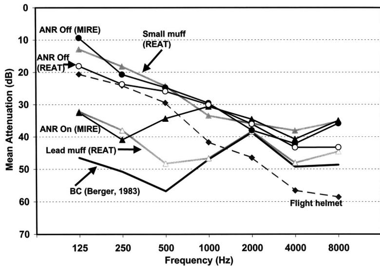
FIG. 4. Attenuation of the ANR earmuff and flight helmet, worn individually, from this study, compared to the muffs from Berger (1983). For the ANR earmuff both real-ear attenuation at threshold (REAT) and microphone-in-real-ear (MIRE) data are compared.
