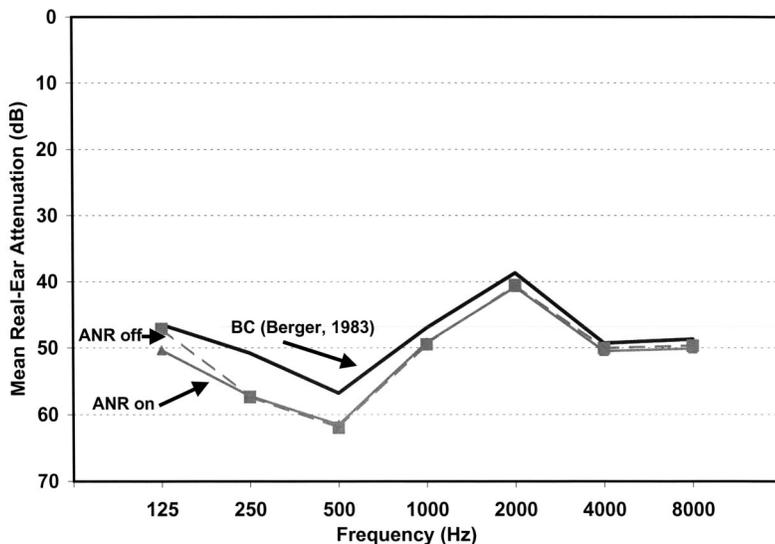
FIG. 8. Real-ear attenuation of the ANR earmuff worn in combination with a deeply inserted foam plug (DI), with the ANR turned on or turned off, as compared to Berger’s (1983) prior BC estimates.
