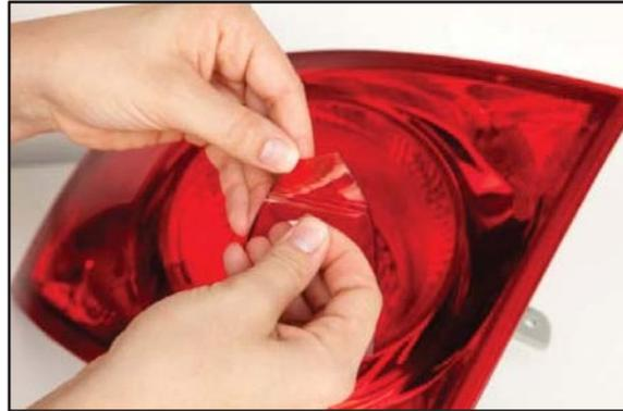
5. Press firmly and evenly across all areas of the film to ensure good adhesion and prevent moisture and dirt from entering the lamp.
