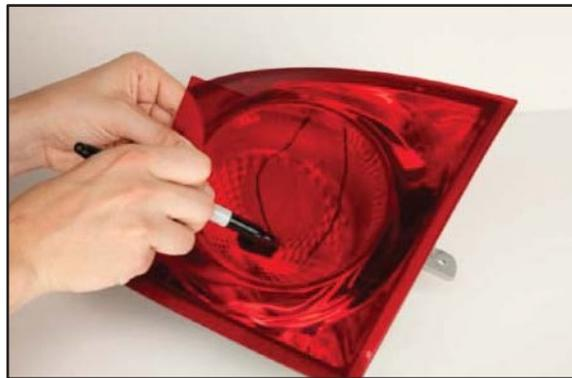
3. Using scissors cut the film to size. Hold the cut piece up to the damaged area before removing backing to ensure correct size. **Note:** For curved surfaces, before removing backing, roll and shape the film in your hands for 60 seconds. This will help form the film to the curve prior to installation.
