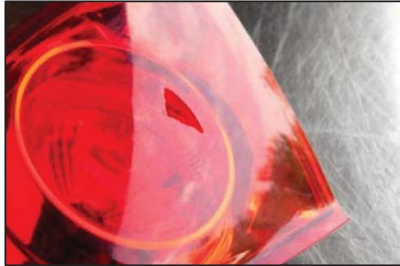
2. The repair film should be cut large enough to overlap the repair by about 1/2 inch on all sides to ensure good adhesion of the film. Hold the repair film up to the damaged area and lightly trace the amount of film needed for the repair with a marker.
