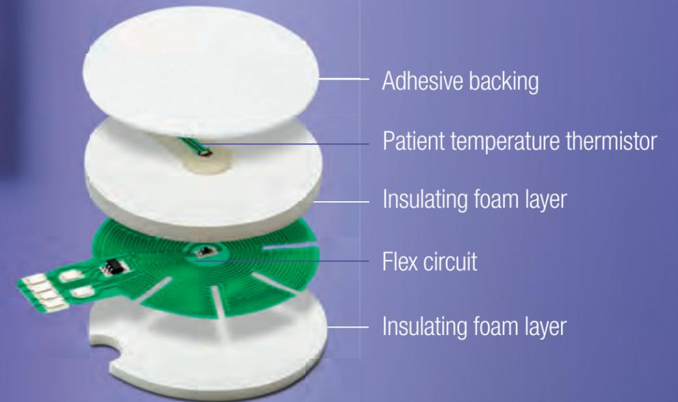
Unlike passive skin surface temperature sensors, the SpotOn system's single-use sensor consists of a thermal insulator adjacent to the skin which is covered by a flex circuit. Once connected to the SpotOn control unit, the flex circuit actively regulates its temperature to create a zone of perfect insulation - a condition where heat loss to the environment is eliminated.
