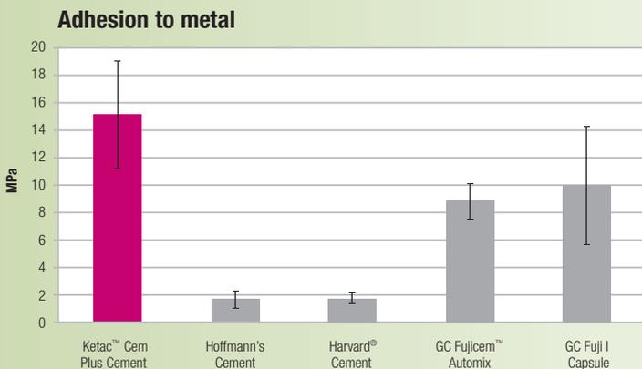
Fig. 7: Shear bond strength to metal. Source: Y. Wang, T. Ton, A. Falsafi, J.D. Oxman, E. Popp, and T. Tran: Adhesion of Glass-Ionomer and Zinc Phosphate Cements to Different Substrates, J Dent Res 92 (Spec Iss A): 2379, 2013 (www.dentalresearch.org).
