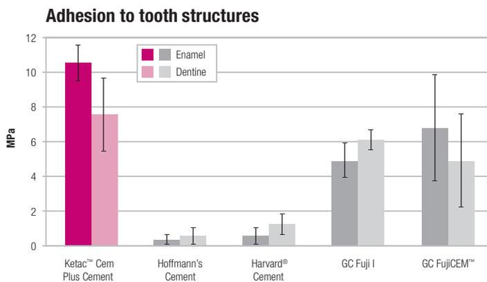
Fig. 6: Shear bond strength to tooth structure, cements used without conditioner. Source: Y. Wang, T. Ton, A. Falsafi, J.D. Oxman, E. Popp, and T. Tran: Adhesion of Glass-Ionomer and Zinc Phosphate Cements to Different Substrates, J Dent Res 92 (Spec Iss A): 2379, 2013 (www.dentalresearch.org).
