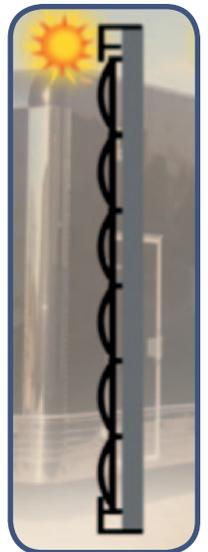
*Mechanically fastened panels can take on a distorted quilted appearance when exposed to heat.*
