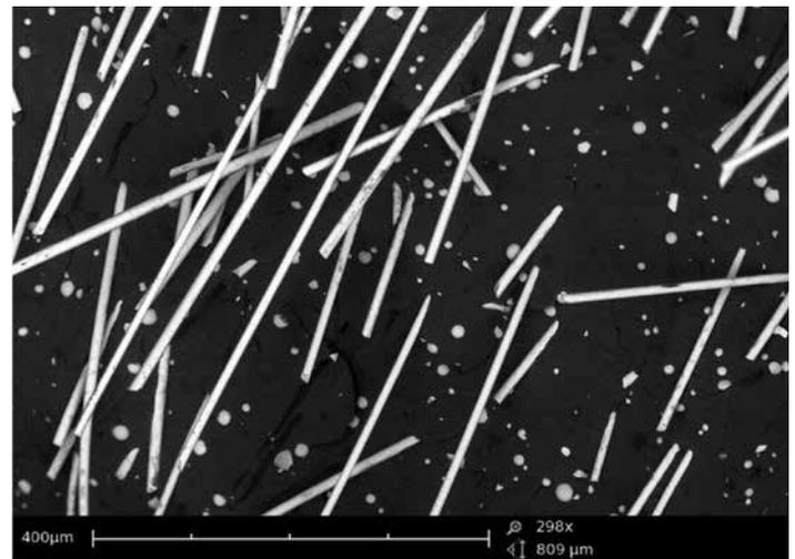
**Figure 3.** SEM image of 19 wt% glass fiber, 10 wt% glass bubbles iM16K in PP
