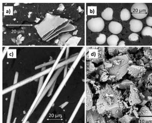
**Figure 1.** Scanning electron microscopy images: a) talc; b) glass bubbles; c) glass fibers; and d) calcium carbonate.
