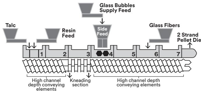
**Figure 2.** Compounding Set-up
