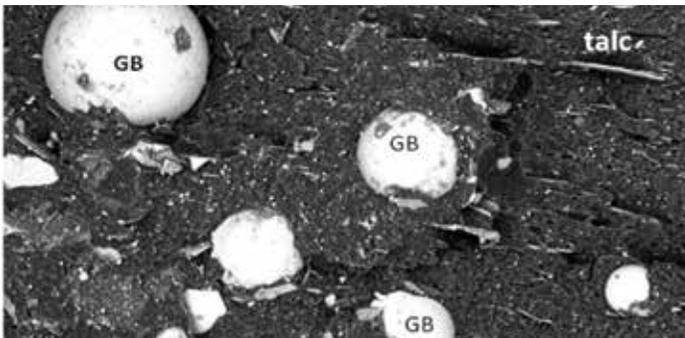
**Figure 5.** SEM image of PP with 10 wt% talc and 4 wt% glass bubbles
