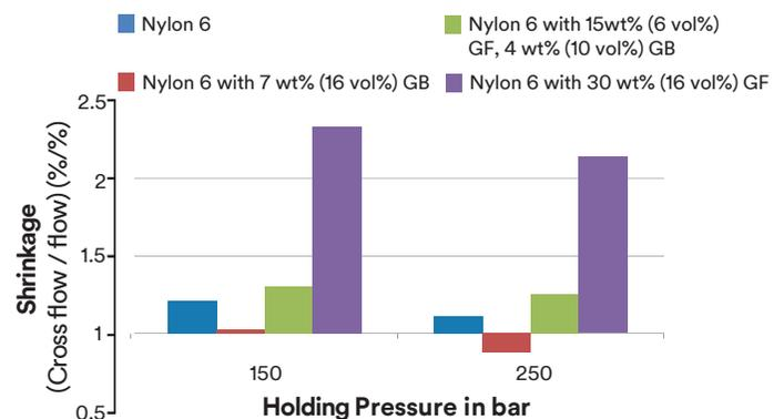
**Figure 7.** Differential Mold Shrinkage
