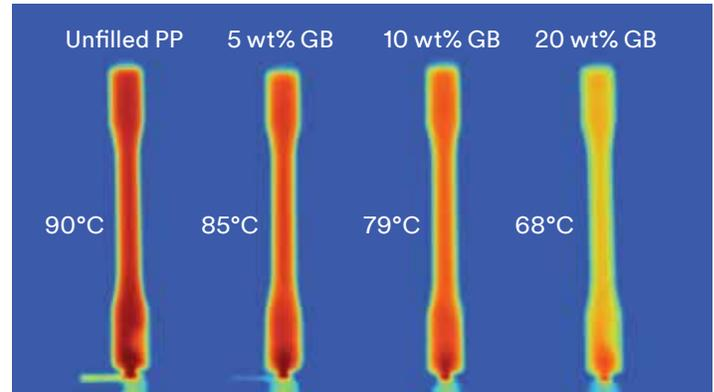
**Figure 6.** Thermal images of molded PP parts containing various loadings of 3M™ Glass Bubbles iM16K. Images taken 15 seconds after part ejection.
