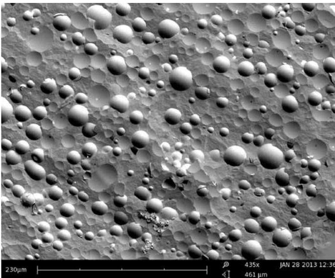
**Figure 3.** SEM image of PP with 10 wt% talc and 4 wt% 3M™ Glass Bubbles iM16K
