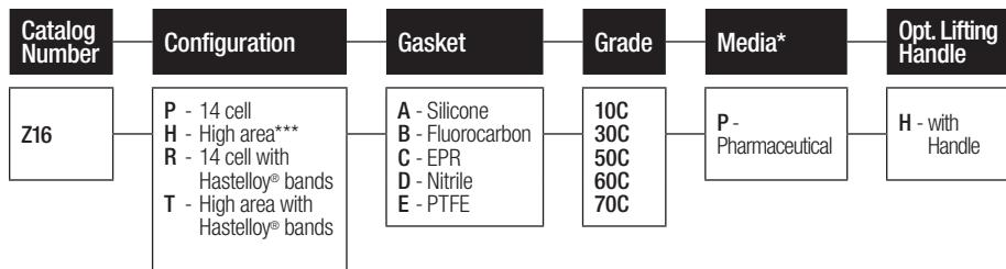
\*Omit "P" from part number for standard C media. \*\*Omit "H" from part number if lifting handle is not required.
