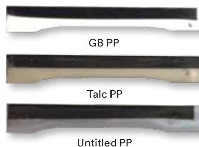
Setup showing adhesive tape with a known thermal emissivity on the tensile bars in order to determine thermal emissivity of parts with different formulations.
