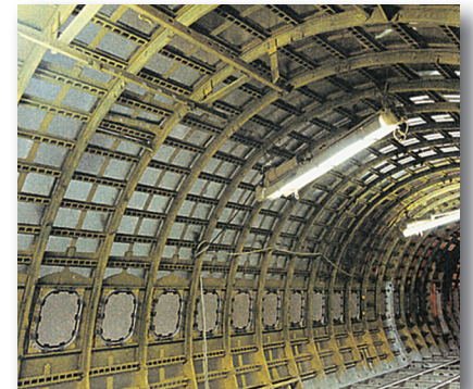
3M™ Damping Foil 435 between the ribs and stringers of an aircraft fuselage helps reduce vibrational fatigue and noise inside the passenger cabin.
