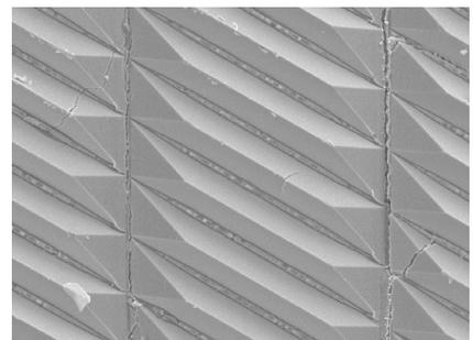
For an even finer sand scratch, elongated distributed abrasive structures are used to provide uniform patterns and consistent sand scratches. This allows for faster buffing and better finishes.
