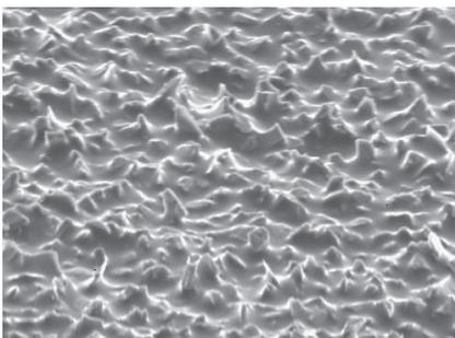
Variable and sized randomly arranged minerals leave inconsistent finish with deep scratches that are hard to buff.
