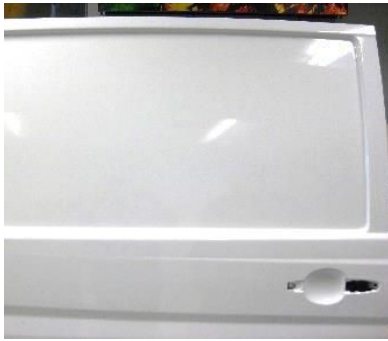
Single Recess using application method "B": Heat stretch - minimum of 20 cm (8") away from recess.
