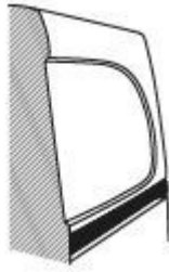
Single Recess using application method "B": Heat stretch - minimum of 20 cm (8") away from recess.
