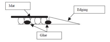
When gluing on edging, solid top of mat faces up and coils face down as shown in the figure above. Recommended maximum edge length is 12 feet (3.6 meters).
