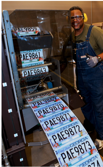
Blanking Line Operator pictured with 3M Sheeting Applicator. Finished license plate sheeting is being applied to aluminum blanks at this station.
