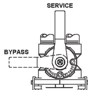
**Figure 4. BYPASS VALVE**
