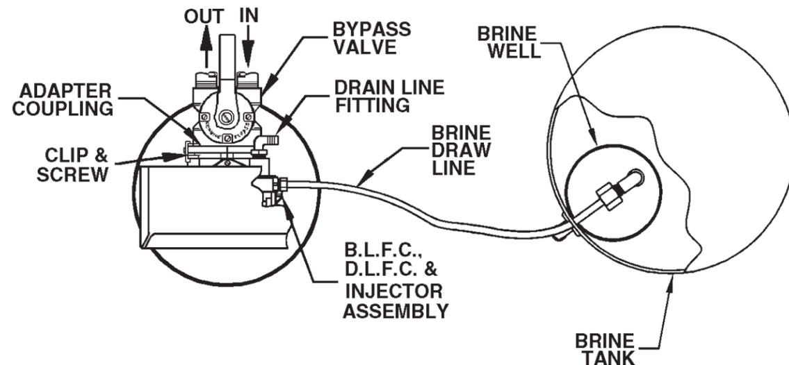
Figure 2. SOFTENER AND BRINE TANK ASSEMBLY, TOP VIEW
