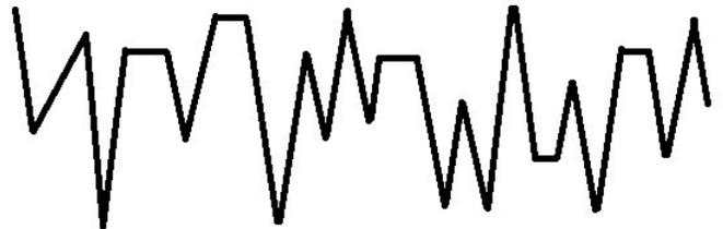
The scratch pattern above is inconsistent and will have an  $R_z$ , and  $R_{max}$  greater than the scratch pattern shown below.
