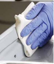
Use a clean cloth or paper towel to clean repair area with 3M™ All Purpose Cleaner and Degreaser followed by a VOC compliant wax and grease remover. DO NOT spray or saturate seams with cleaner.
