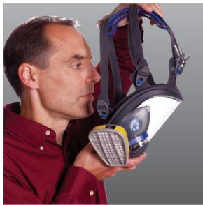
Fully loosen all six head straps. Hold the front of the facepiece with one hand and the straps/comfort cradle away from the facepiece with the other hand, creating an opening for the head. Pull the respirator assembly down over the head. Place the nose in the nose cup and chin in the chin cup area then press the facepiece firmly and evenly against the face.
