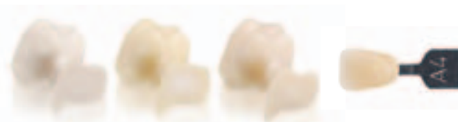
Fig 5: Color match comparison of A4 shaded 3-unit bridge frameworks cut through the connector. From left to right: Competitor 1, Competitor 2, Lava™ Plus Zirconia, VITA classical shade guide.
