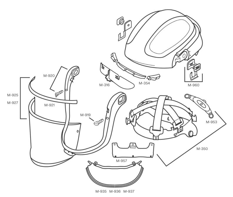
If you discover any signs of wear and/or damage, remove headgear from use and service or replace as appropriate. 3M recommends a maximum life (shelf life plus in use life) of 5 years from the date of manufacture. See the M-Series User Instructions for details on inspection and replacement.
